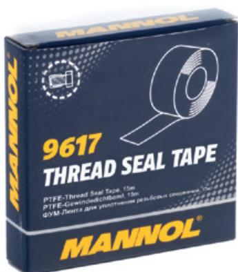
**EN** Universal PTFE tape for sealing threaded connections ("foam tape") of any material (metal and plastic, etc.). It can be used both in the repair of cars and other equipment, and in industry and everyday life when installing and repairing plumbing units and gas pipes. Product properties: length/width/thickness – 15m/19mm/0.075mm; low coefficient of friction. Fluorine - containing plastic polymers (PTFE) have a very low coefficient of friction, which facilitates the connection of fittings.
